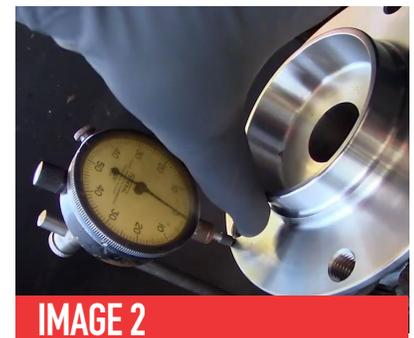
**This is an important reminder not to make quick assumptions. When doing a brake job, always perform a thorough brake inspection list, which includes checking the wheel bearings for significant play.**
