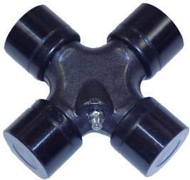
U-Joints include nitrile rubber seals, which offer premium quality grease retention and contaminant resistance. Bearing caps are also induction heated and hardened only on the race surface to produce a flexible, yet durable steel, which allows for easier installation into tight yoke tolerances.
