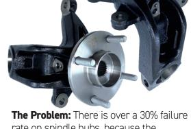
**The Problem:** There is over a 30% failure rate on spindle hubs, because the bearing race often seizes to the hub and cannot be separated
