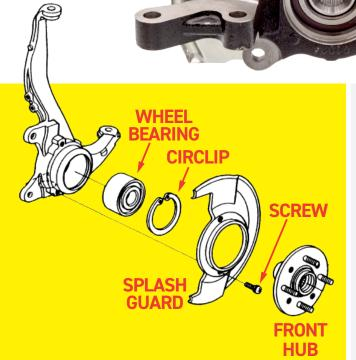
**THE PROBLEM:** There is over a 30% failure rate on spindle hubs due to a damage from road hazards, collisions, or rust accumulation which causes the bearing race to seize to the hub and cannot be separated
