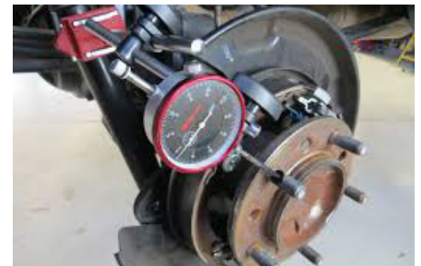
Use a dial indicator to measure runout as part of every brake job
