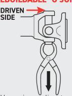
• Use a vise or pliers to remove the bearing cap which is exposed on the opposing side. Use a twisting motion to help unseat the cap.
