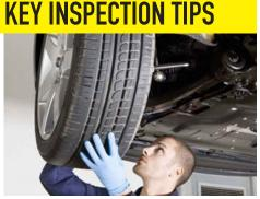
1. Check for early warning signs of a worn bearing which may include friction noise on wheel rotation, or an unusually slow turning wheel when suspended on a rack.
