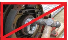
8. Never use a hammer to hit directly on the bearing.
