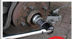
9. Manually torque the bearing nut to the correct OE specified preload.
