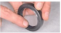
7. Check the contact surface for the seal lip. Even the smallest mark or rust will damage the seal lip and allow water penetration and eventual corrosion.
