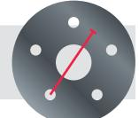
Aother way to measure the odd number bolt pattern is by measuring the center of a stud to the center of the next stud. The measurements for the 5 hole patterns:
