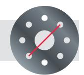
On hubs with an odd number of studs, measure any stud center to the point halfway across between studs on the unit. Example: 5 on 4-1/2" would mean 5 bolt holes with 4-1/2" measure to a point halfway between the opposite studs.
